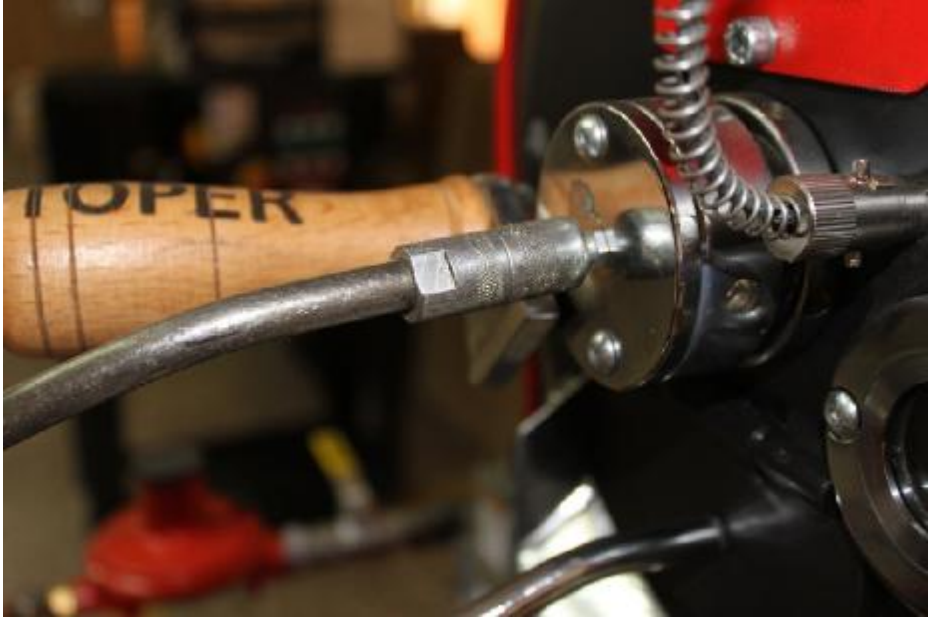
Figure 24 The front of the drum adjustment cover should be lubricated as well with the oil pump
