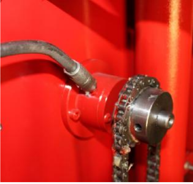
Figure 22 In order to lubricate the drum back bearing, please remove the motor housing by using Allan Key.Lubricate the point as shown in the figure with the oil pump. Figure 23 Note: Fort his aplication please use Mobiltemp SHC 460 Special grease oil or like the sama speficitaions.
